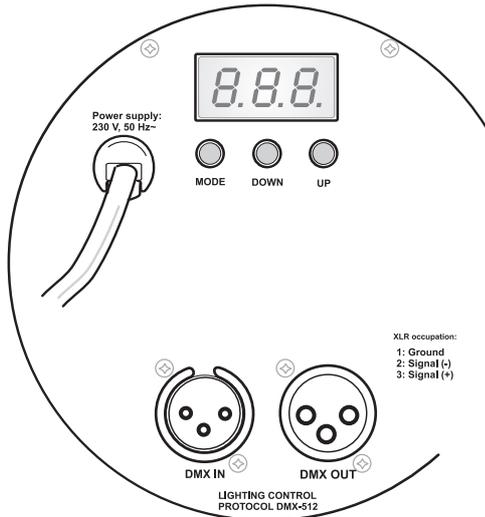
The Control Board offers several features: you can run the internal programs or set the starting address.
